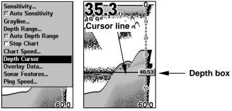
Sonar Page menu with Depth Cursor command selected (left). Sonar chart with the depth cursor active (right). The line indicates the large fish is 40.53 feet deep.
